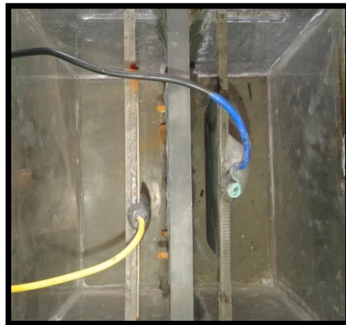
Figure 2: Top view of MEC (with lid open) showing the electrodes with and arrangement to adjust spacing between the electrodes
