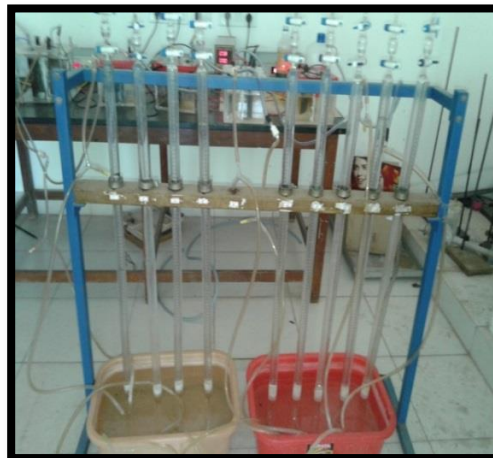
Figure 4: An arrangement to collect gases using burettes by downward displacement of water
