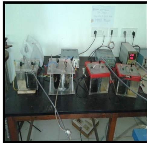
Figure 3: MECs filled with waste water in anode chamber and distilled water in cathode chambers with electrodes connected to an external power supply
